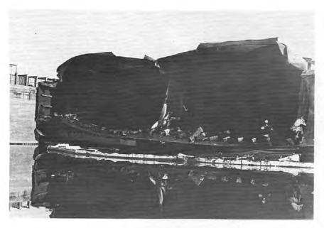
pairs being undertaken on a tank barge that was not gas free. This resulted in the ignition of vapors from cargo and cargo residue in the No. 1 starboard wing void which spread fire throughout the forward section of the vessel and ignited volatile vapors causing an explosion. The disregard for federal regulations and unsafe practices on the part of the marine chemist and the owners of the vessel resulted in this fatal accident.
