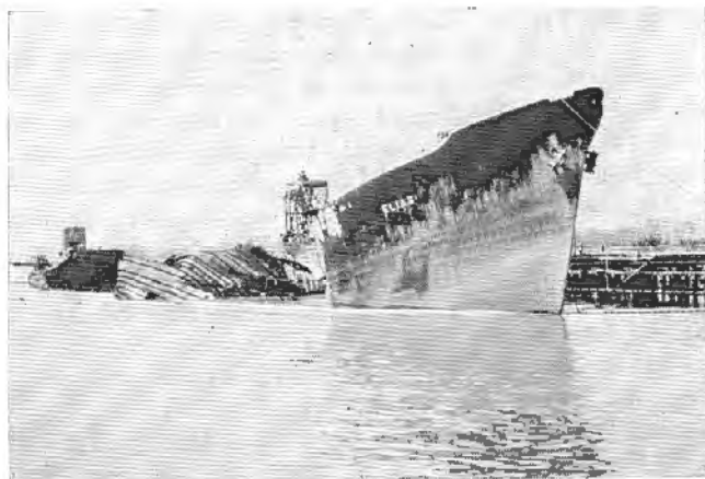
Could a cargo tank inerting system have prevented this casualty? These views of the crude oil carrier Elias show the massive damage caused by the explosions and fire which erupted during the offloading process. Thirteen persons were killed in this casualty, which occurred just before midnight on 9 April 1974.
