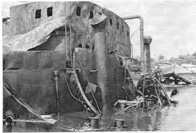
Could a cargo tank inerting system have prevented this casualty? These views of the crude oil carrier Elias show the massive damage caused by the explosions and fire which erupted during the offloading process. Thirteen persons were killed in this casualty, which occurred just before midnight on 9 April 1974.
