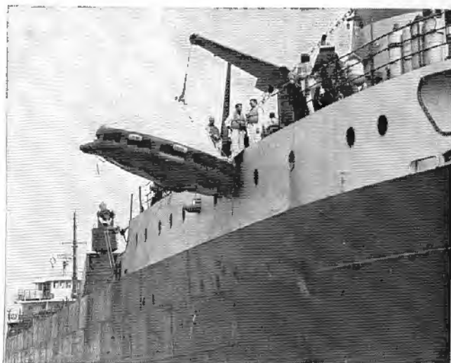
Two methods of personnel evacuation are shown undergoing tests in these photos. On the left a davit launched inflatable liferaft is being examined on board the M/V Joseph Frantz . A winter test of an inflatable evacuation slide in Lake Superior is shown in the photo at right.
