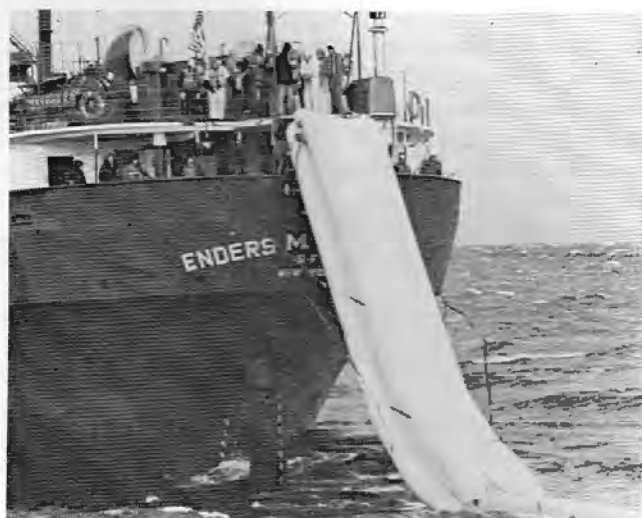
Two methods of personnel evacuation are shown undergoing tests in these photos. On the left a davit launched inflatable liferaft is being examined on board the M/V Joseph Frantz . A winter test of an inflatable evacuation slide in Lake Superior is shown in the photo at right.
