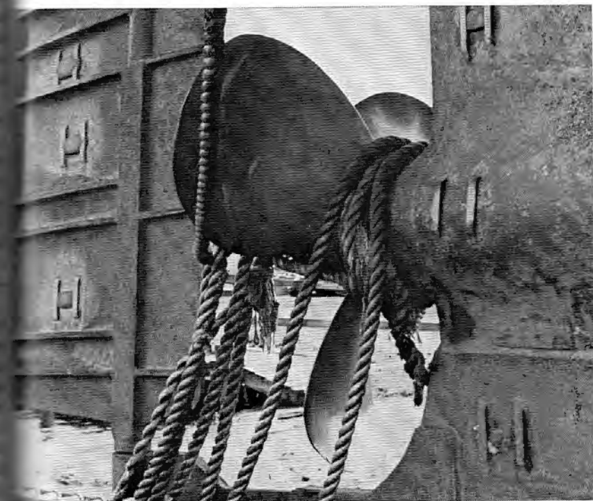
The unused section of the towing hawser washed overboard as the Grayland attempted to cross Albemarle Sound. When the tug stopped to lengthen the towline, a loose bight fouled the propeller as shown above.
