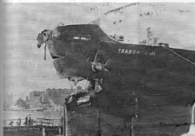
The above photos show the extent of the bow damage incurred by the SS Transhawaii . Repairs were made in Baltimore.
