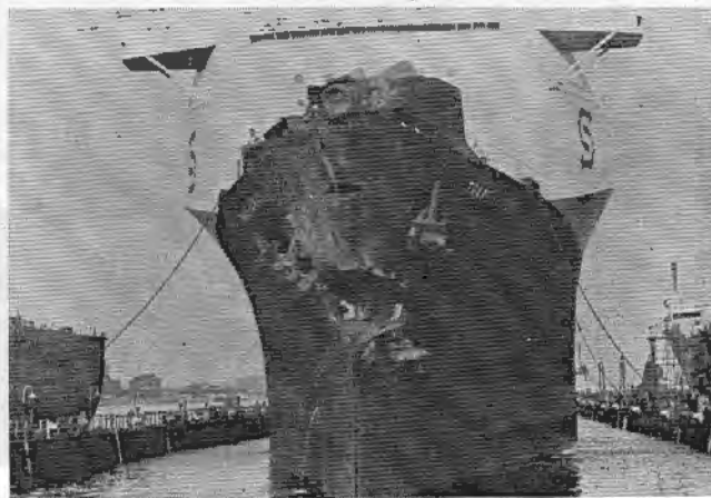
The above photos show the extent of the bow damage incurred by the SS Transhawaii . Repairs were made in Baltimore.
