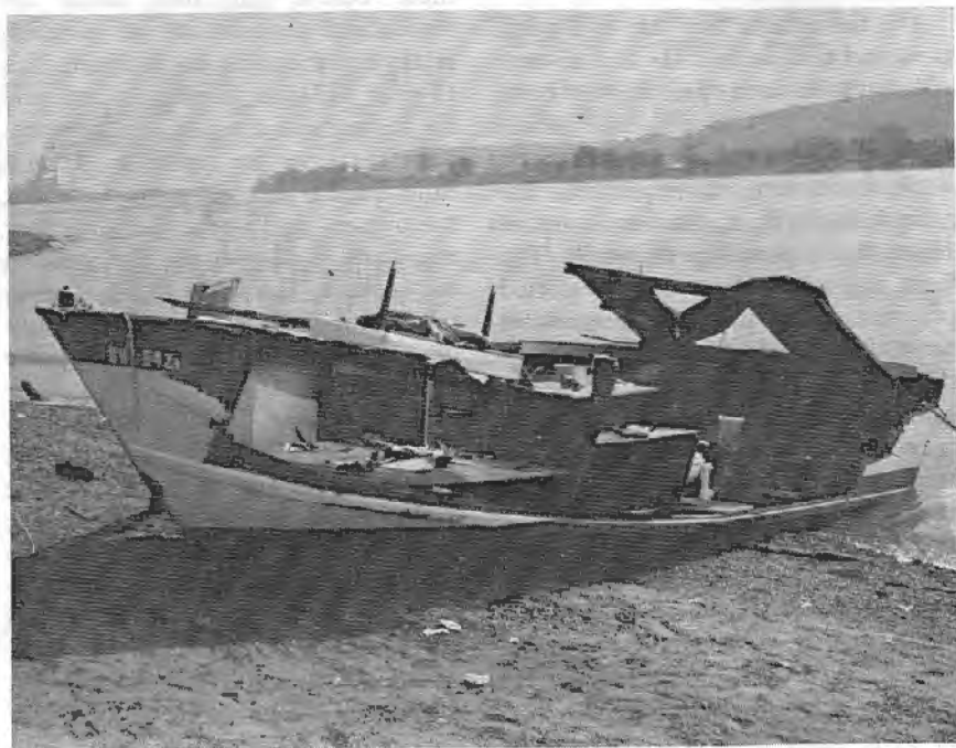
Although the pleasure boat was struck on the starboard, greater damage was done to its port side as the boat was pushed over and tumbled beneath the barges.
