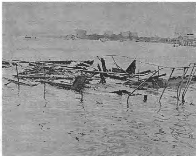
This can be the result when a source of ignition and gasoline vapors meet aboard a recreational boat. It is hoped that regulatory standards will help eliminate such sights.
