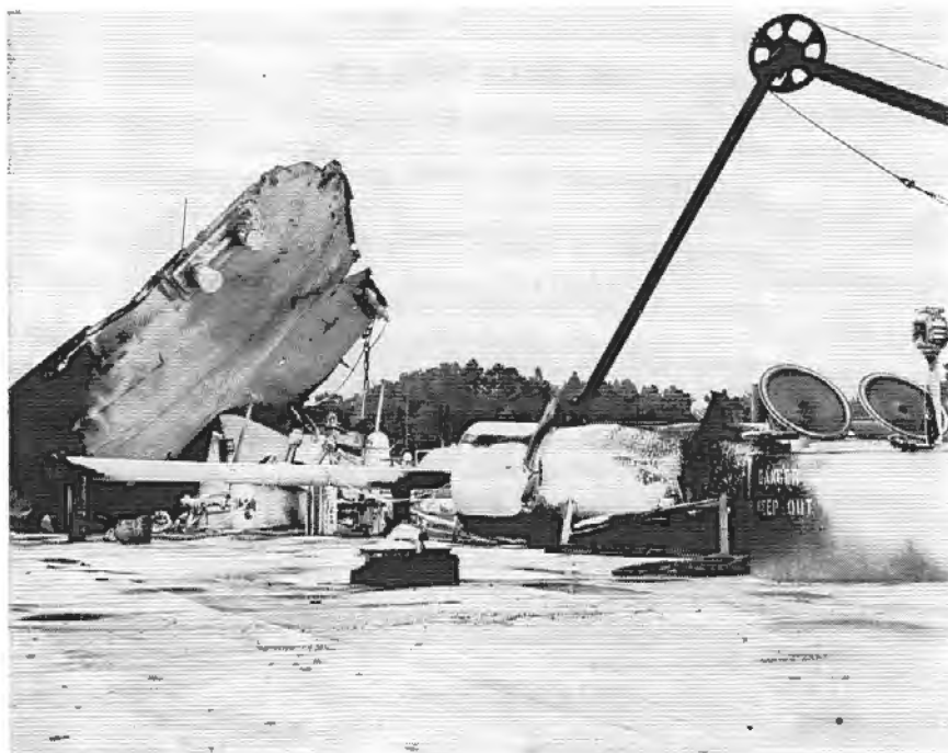
The above photograph was taken from the starboard side of the Sun Chem 1100's deck, looking aft. It shows the expansion trunk to the No. 3 port and starboard tanks, the manifold, and much of the damaged area. The rigging at the top right is the shore side connection to the manifold on the barge.
