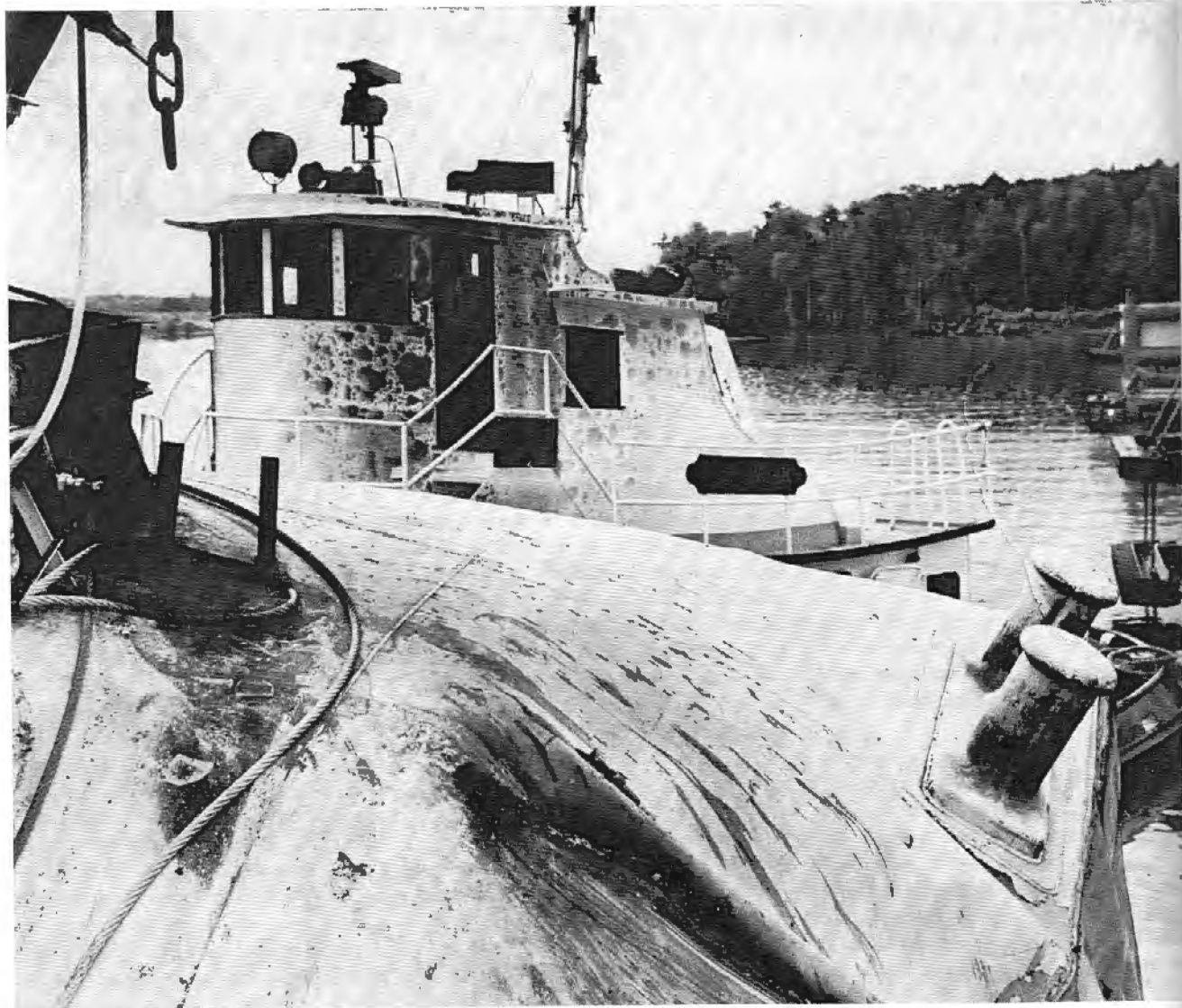
The New Work was scorched by the fire in the alternate route of the Gulf Intracoastal Waterway, but otherwise she remained seaworthy and was able to push the still watertight Sun Chem 1100 to Port Arthur, Tex., for repairs.
