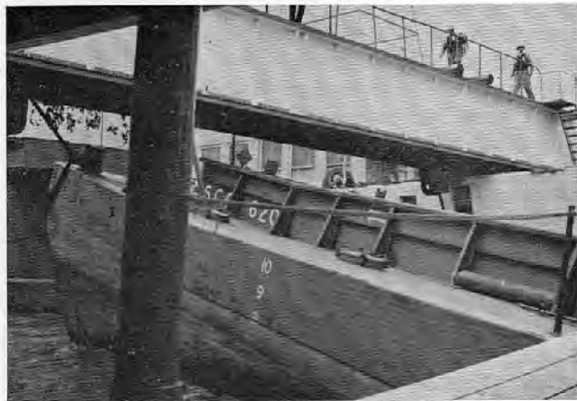
A salvage contractor's catamaran constructed of two World War II patrol craft hulls joined by a crossbeam provided both a stable working area and an important anchor for the chlorine barge. These pictures indicate how the unique craft was used to straddle SCC 620 and hold it in place by means of a wire rope sling passed under the barge's bow.
