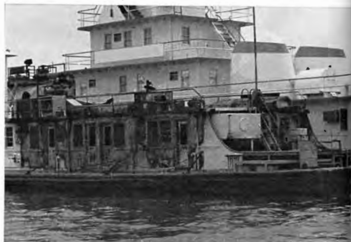
These two views of the M/V Martin show the burned-out galley (at the stern) and adjoining spaces.
