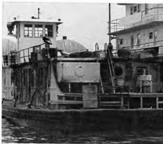
These two views of the M/V Martin show the burned-out galley (at the stern) and adjoining spaces.
