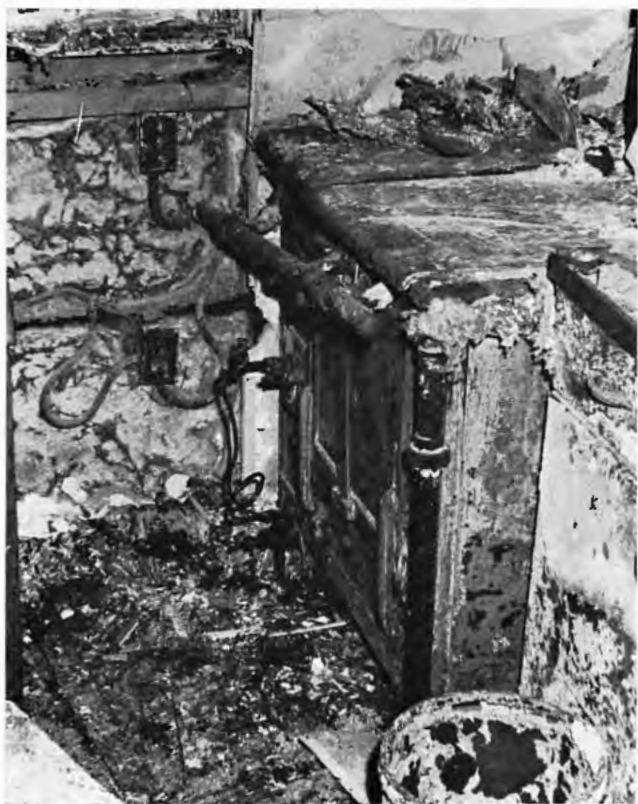
This interior view taken 2 days after the incident, shows the scorched remains of the oil-fired galley range on the M/V Martin .
