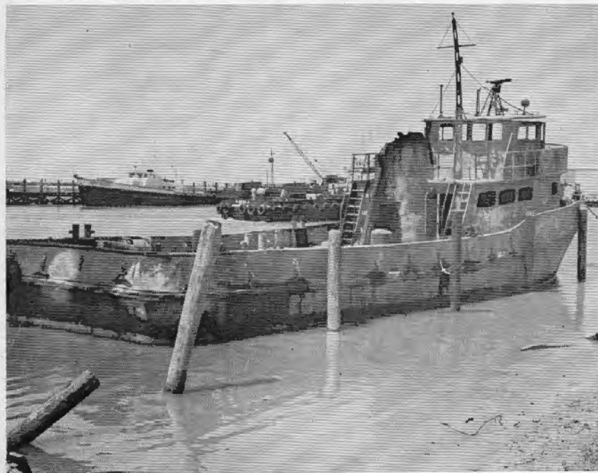
The M/V Carryback is shown gutted and scorched moored at Galveston, Tex. where she was towed after the casualty.
