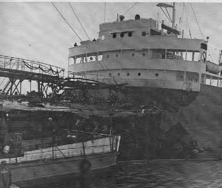
When the vessels were separated, the damage to the Oregon Standard looked like this. Ullage trunks and external fittings on the deck area were sheared when the overhang of the Arizona Standard's bow slid aft on the Oregon Standard. Heavy bunker oil from the three ruptured cargo tanks spilled into the San Francisco Bay, causing extensive pollution damage.
