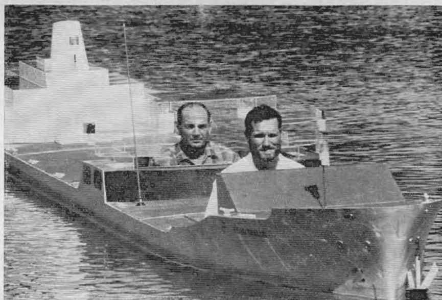
The two-man Esso Berlin is 26 feet in length and is a 1/25th scale model of its 38,000 ton namesake. The training center has facilities in the same 1 to 25 scale as the models. The layout includes a bend in the Suez Canal, two fixed bow mooring towers, a floating mooring buoy, two conventional buoyed sea berths, and lighted buoys to make channels.
