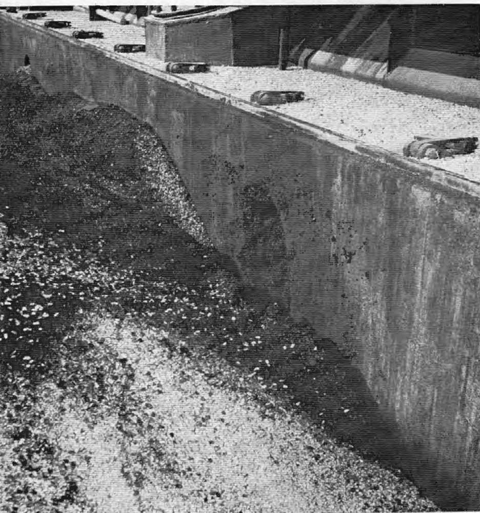
FIGURE 4. Source of fire may have been a result of hold flood lights being left on after the cargo of corn was loaded. Note charred grain in recess of flood light.
