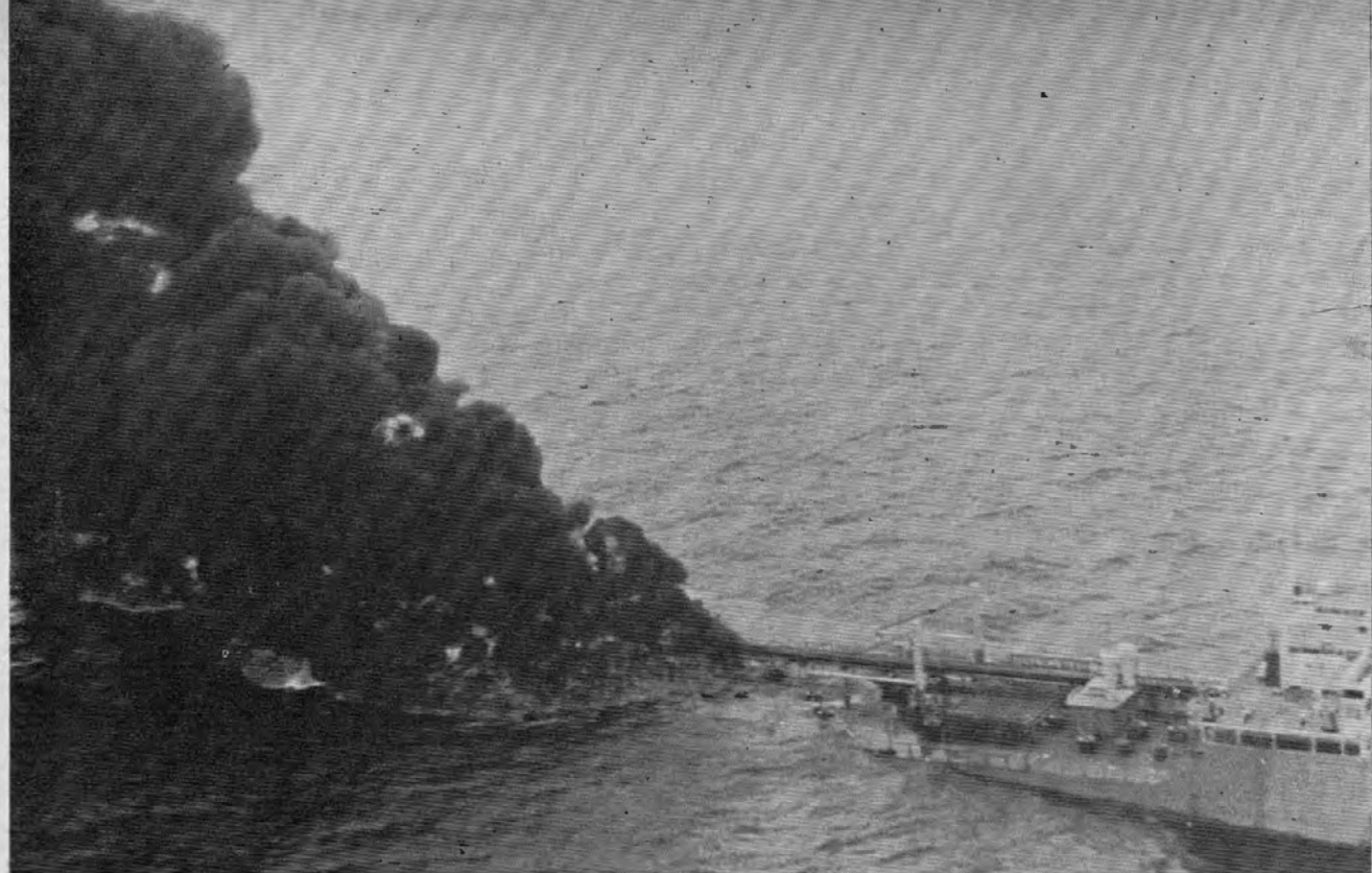
Aerial photo taken by Coast Guard HU-16E aircraft showing Gulfstag down by the stern, after main deck awash with after house engulfed in flames.
