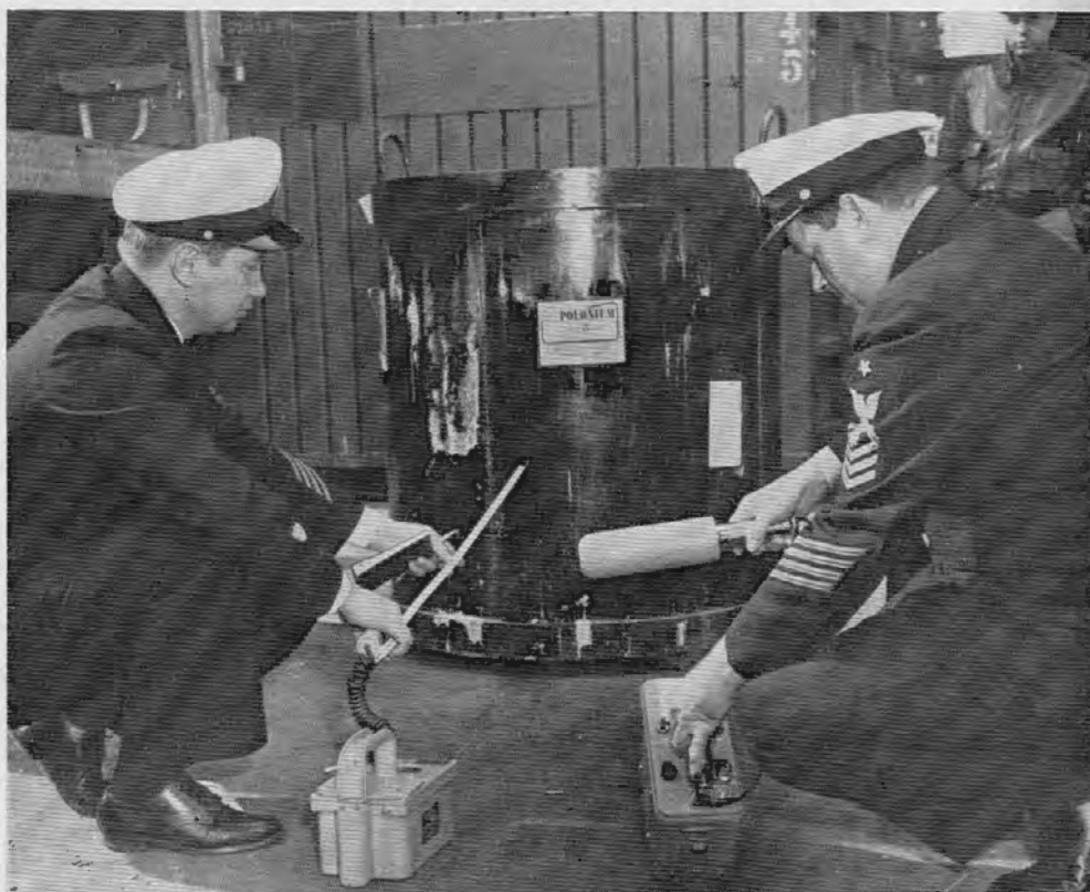
THE CAPTAIN of the Port dangerous cargo team verifies that the radiation from a radioactive materials package is within safe limits.
