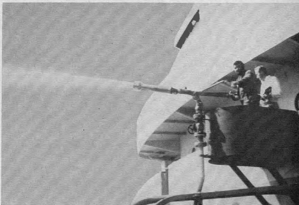
A PC-50 monitor station, discharging foam solution at a rate of 500 g.p.m. This station is a part of a foam system used aboard the Mobil Acme .
