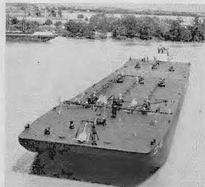
A SULPHURIC ACID BARGE fitted with six cylindrical and integrated cargo tanks.
