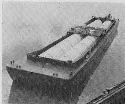
INDEPENDENT TANK BARGE for chlorine service showing the arrangement of tanks in the hopper space.
