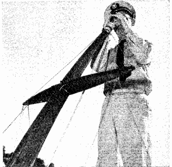
AS CERTAIN LIGHTS MUST be displayed on a motorboat between sunset and sunrise, the Examiner checks to see that they are operating and will show within the prescribed sectors.
