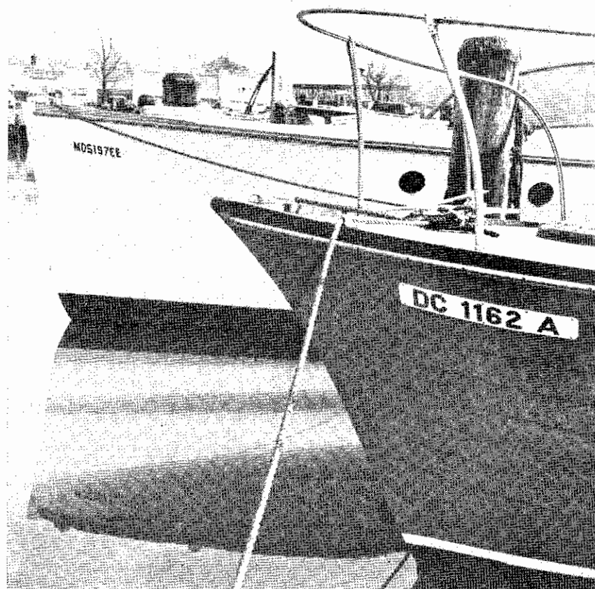
THE BOAT on the left displays a registration number which is incorrect—the symbols are too close together and there is no spacing between the letter groups and the numbers. The boat on the right displays correct spacing of the letters and numbers.
