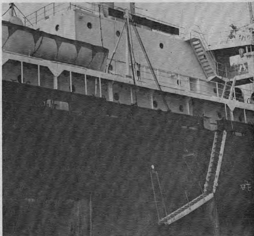
A LIBERTY SHIP gangway supported by a boat fall. This practice resulted in a shipmaster having his license suspended for 4 months for failure to have the lifeboat available for use while at anchor.
