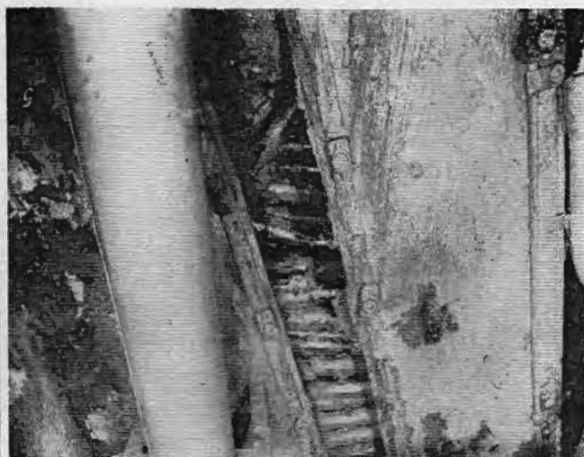
LOOKING AFT in the port boiler furnace. Burner openings at left, melted tubes at right.
