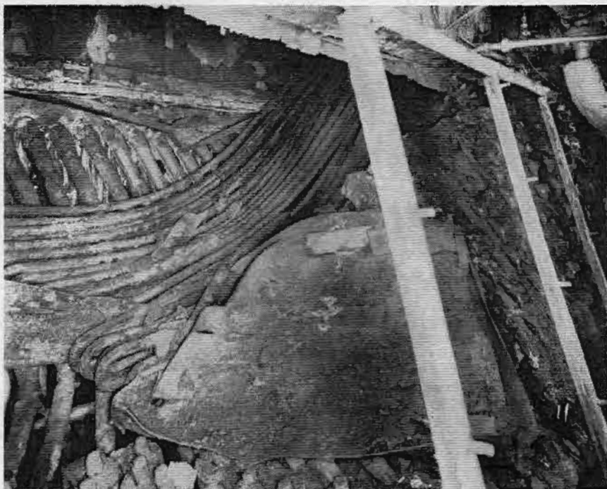
REAR VIEW of the port boiler which shows collapsed headers, recirculating tubes, and superheater tubes.
