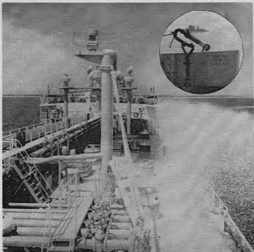
DURING RECENT SEA TRIALS OF THE "JUMBOIZED" SS Fort Fetterman a group of interested industry and government officials witnessed a test of the newly installed deck foam system seen in this photograph. Photo Courtesy Keystone Shipping Co.
