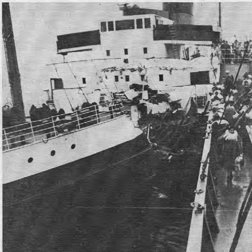
Figure 3. View of forward section of Duke of York shortly after collision. The section forward of the point of impact broke off and sank. Survivors can be seen on the foredeck of the Haiti Victory .
