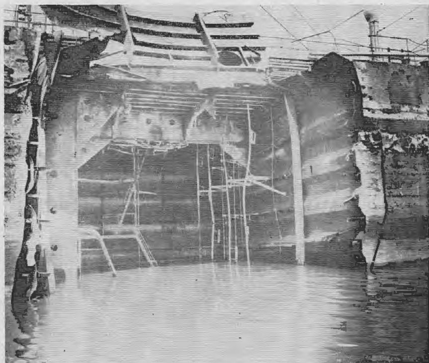
Figure 3. Inboard view of the SS Esso Paterson showing extent of explosive force which catapulted bulkhead between No. 8 port and No. 8 center tanks almost 100 feet from the ship.
