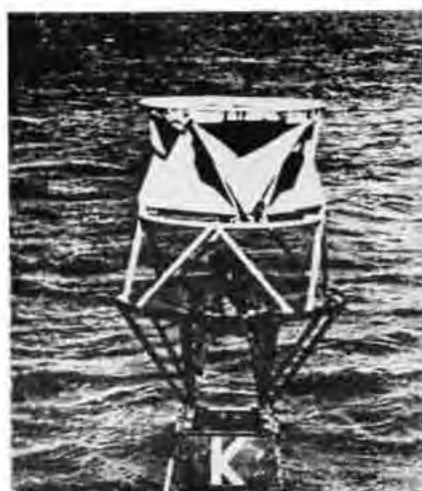
Figure 6.—Radar Reflector Cluster Mounted on Lighted Buoy.
