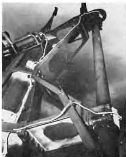
FIGURE 5.—Photograph showing grease lines on periscope structure of a submarine.
