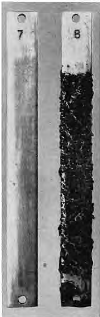
FIGURE 1.—Comparison of the rusting on steel strips which have been immersed in inhibited and noninhibited turbine oils for the 48-hour test.
