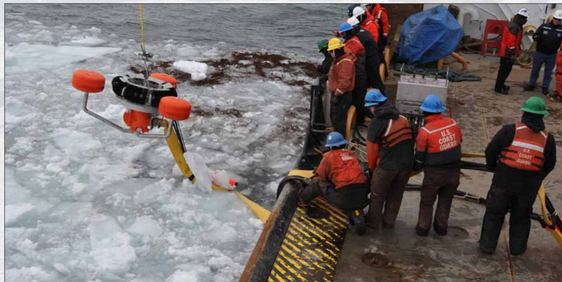
Crewmembers aboard the Coast Guard Cutter Hollyhock use an oil skimmer to recover peat moss, acting as a substitute for spilled oil, near Mackinac Island, Jan. 24, 2012.
