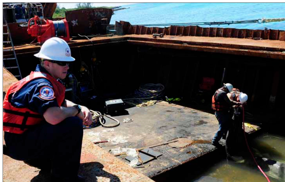
Petty Officer 1st Class Kenny Cook, with the Atlantic Strike Team, supervises as response crews insert roller bags in the 202-foot grounded freighter Jireh Sept. 3, 2012 to prepare the vessel for final removal and disposal. U.S. Coast Guard photo by Petty Officer 1st Class Crystallynn A. Kneen.
