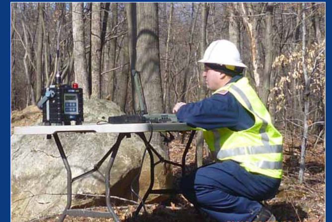
Petty Officer 2nd Class Jonathan Scott conducts air monitoring using a specialized gas meter during excavation operations at the dump site, Feb. 22, 2012. U.S. Coast Guard photo by Petty Officer 1st Class Seth Hartmann.
