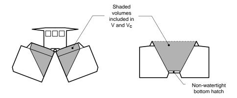
R.6(3)-3 Spaces open to the sea should not be excluded from the total volume of all enclosed spaces (V) if they are used for cargo and/or buoyancy purposes.
