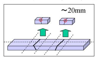
Figure App 3 - Sectioning plan
