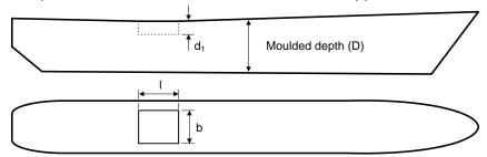
R.2(1)-4 In a ship having openings in the side of the ship below the uppermost deck, which are not closed but limited inboard by weathertight bulkheads and decks, the deck below such openings should be considered the upper deck.
