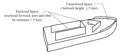
In the situation where only a portion of a bulkhead or partition exceeds 5 feet (1.5 meters) in height, the entire inboard space in way of that portion of the structure from the deck to the top of the structure must be included in the total volume of all enclosed spaces (V).
