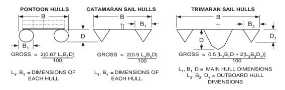
(4) If the volume of the principal deck structure of a vessel is as large as, or larger than, the volume of the vessel's hull, the volume of the principal deck structure in tons of 100 cubic feet is added to the tonnage of the hull to establish the vessel's gross tonnage. The volume of the principal deck structure of a vessel is determined by the product of its average dimensions.
