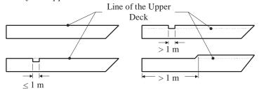
**MOLDED DEPTH** means the vertical distance amidships between the following points:
