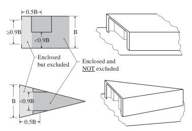
For the situation where the breadth of the space decreases solely due to the convergence of the outside plating, the 90% restriction does not apply.
