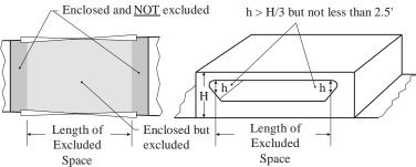
If the opening is only on one side of the deck structure, the space to be excluded is limited inboard from the opening to a maximum of one-half the breadth of the deck in way of the opening
