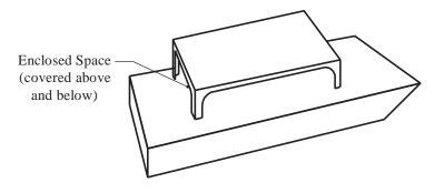
(b) covered from above or below <u>and</u> enclosed on three or more sides by partitions or bulkheads that exceed 5 feet (1.5 meters) in height as measured from the lowest point of the enclosed space.
