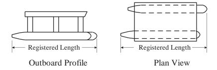
STEM means the foremost boundary of the buoyant hull envelope.
