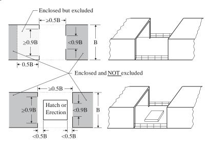
(4) **Determining Breadth of Deck** (B) When the deck at the line of an opening has rounded gunwales, the breadth of the deck is the distance between the tangent points indicate **below**.
