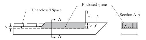
No break (e.g. step) in a deck, nor any opening in the vessel's hull, in a deck or in a covering of a space, or in the partitions or bulkheads of a space, nor the absence of a partition or bulkhead precludes the space from being included in the total volume of all enclosed spaces (V). The following miscellaneous spaces are considered enclosed spaces:
