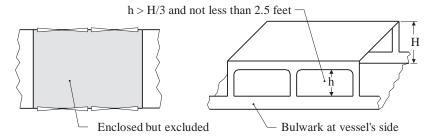
These same requirements apply to the situation where an interior structure partially supports the overhead deck covering.
