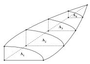
Any mathematical method may be used, provided it accurately models the configuration being measured. Any appropriate area or volume integration method may be used, such as Simpson's First Rule, Trapezoidal Rule, etc. Also, areas or volumes may be integrated along any axis (vertical, horizontal and/or longitudinal) on the vessel as convenient to capture the actual total structure volume.
