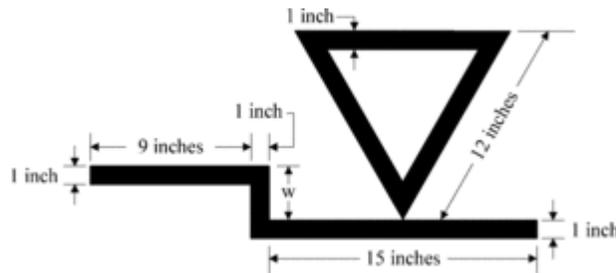
$W = \frac{1}{48}$  of the distance from the top of the flat keel to the tonnage mark. (See §69.177(b)(2).)
