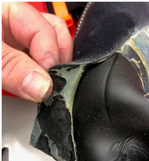
Figure 2: Glue peeled away near the chin area
