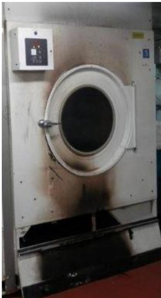
Laundry systems and the normal production of dryer lint create significant fire hazards due to the flammability of the lint. Nearly two decades ago, a fire occurred on a cruise ship due to a welding spark igniting lint. As a result, operators have developed dryer fire prevention procedures that
