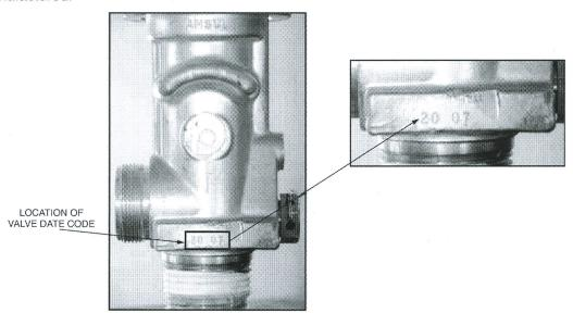
Carbon dioxide cylinders which are installed, or could be installed on a ship with a valve date code between 10-07 and 06-08 **MUST** be identified. If you identify cylinders with valves in this date code range, please contact ANSUL Quality Assurance **IMMEDIATELY** for further information and authorization for replacement of these cylinders.
