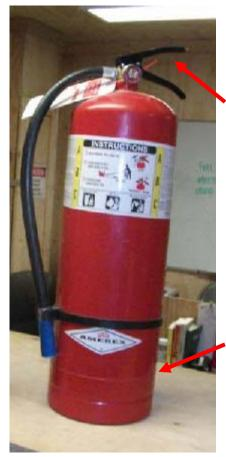
The counterfeit extinguishers have been reported to have black or red plastic handles. Genuine approved dry-chemical B-II extinguishers typically have handles that are constructed of silver-colored aluminum (although there are some with plastic handles).
