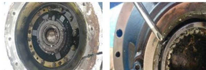
Figs. 5 and 6: Interior of above reduction gears after running in a dry condition leading to overspeed damage
