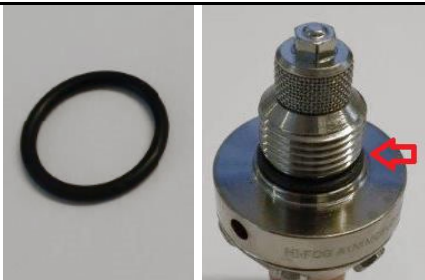
15x2,0 O-ring to replace the 15x1,5 O-ring supplied with sprinklers
