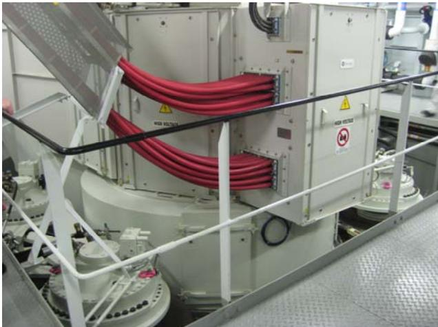
This is another view of the slip ring unit. This unit sits directly over the slewing bearing for the pod. All cables and piping enter the pod at this point.
