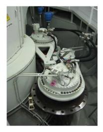
Here is a picture of the two of the hydraulic motors used to rotate (articulate) the pod. There are four motors for each pod, and the pod can operate without reduced capacity with the loss of one motor. The pod can operate with the loss of two motors, but there may be some reduction in maneuverability.
