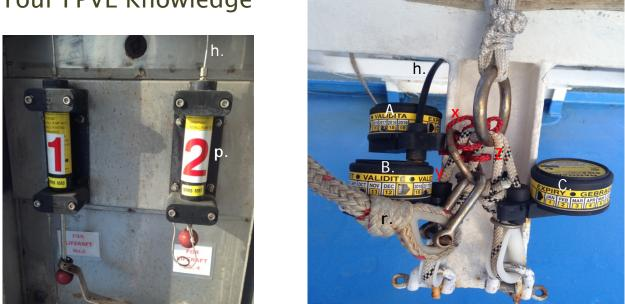
Have you seen a life-raft set up like this before? Do you understand how the system works in order to know if it is installed properly?
