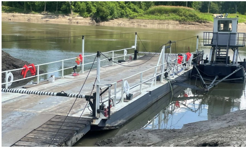
Figure 1. Photograph of deck barge post casualty with recommended bar installation on bow and stern.
