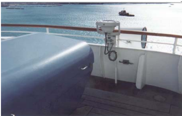
Starboard bridgewing gyro repeater. Note the obstruction in the left foreground.
