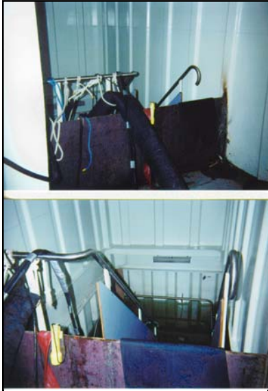
Resultant flooding of stairwell on main deck, port side, forward passageway. Note the welded steel plate across opening to prevent further progressive flooding.
