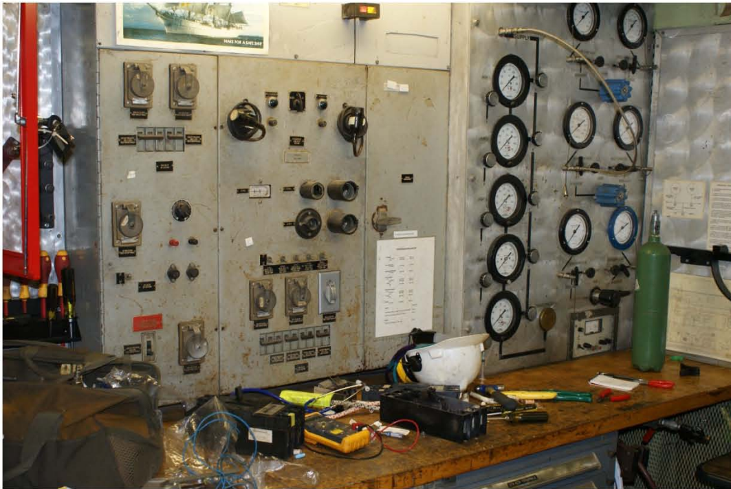
Figure 6: Photograph of the S/R WILMINGTON Electrical Test Panel and Workbench. Note: the test panel also includes a pneumatic testing area (right side).
