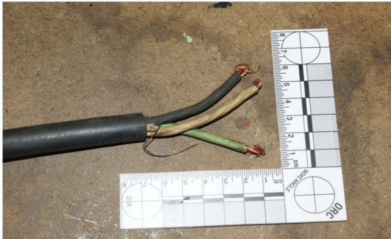
Figure 7: Photograph of the fabricated electrical test lead test lead or "pigtail" consisting of a four (4) prong plug, a six (6) foot insulated cord, and three bare exposed wires.
