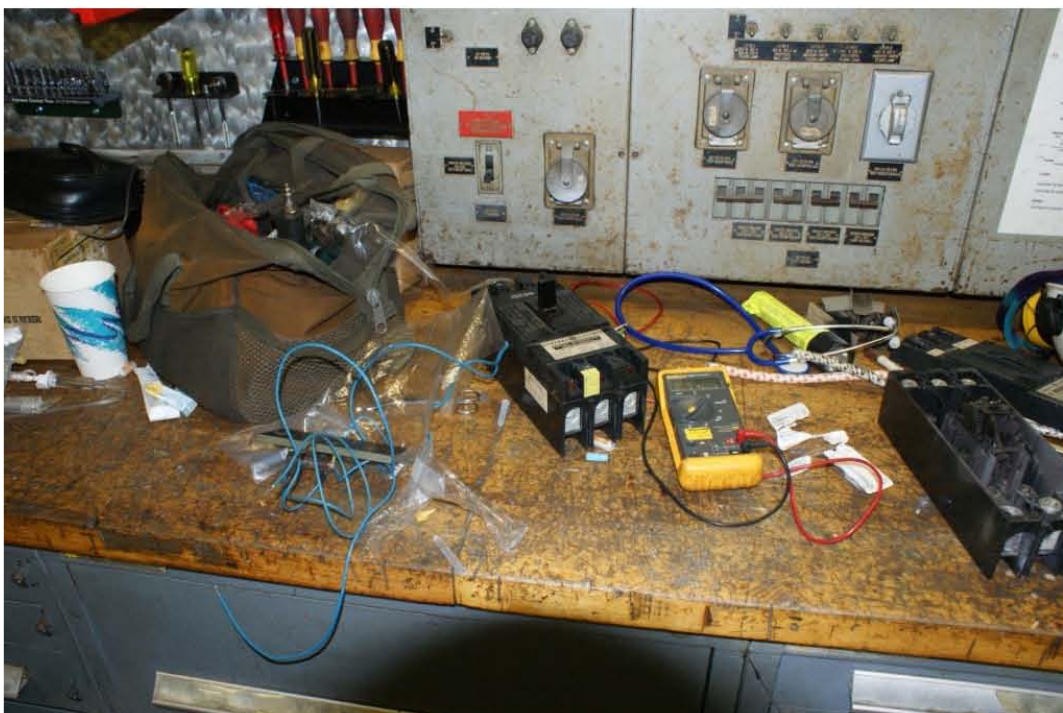
Figure 5: Photograph of the undamaged circuit breaker with the undervoltage release functionality (left) and the damaged circuit breaker (right)
