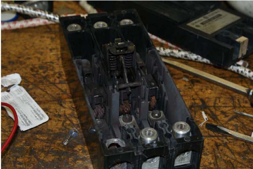
Figure 4: Photograph of Damaged Circuit Breaker
