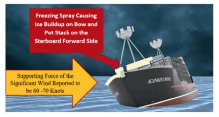
A model showing the final hour of the SCANDIES ROSE with significant icing on the starboard bow and pot stack, leading to the vessel listing into a significant wind on the starboard bow.
