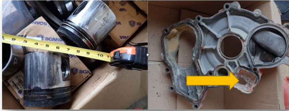
Figure 15 – Damage to PMDE from the initial coolant leak in that engine on May 15, 2022. Left, damaged pistons from the overheating event necessitating a top end overhaul of the engine. Right, arrow points to hole in the water pump cover caused by internal corrosion. (Source: Bay Diesel & USCG)
