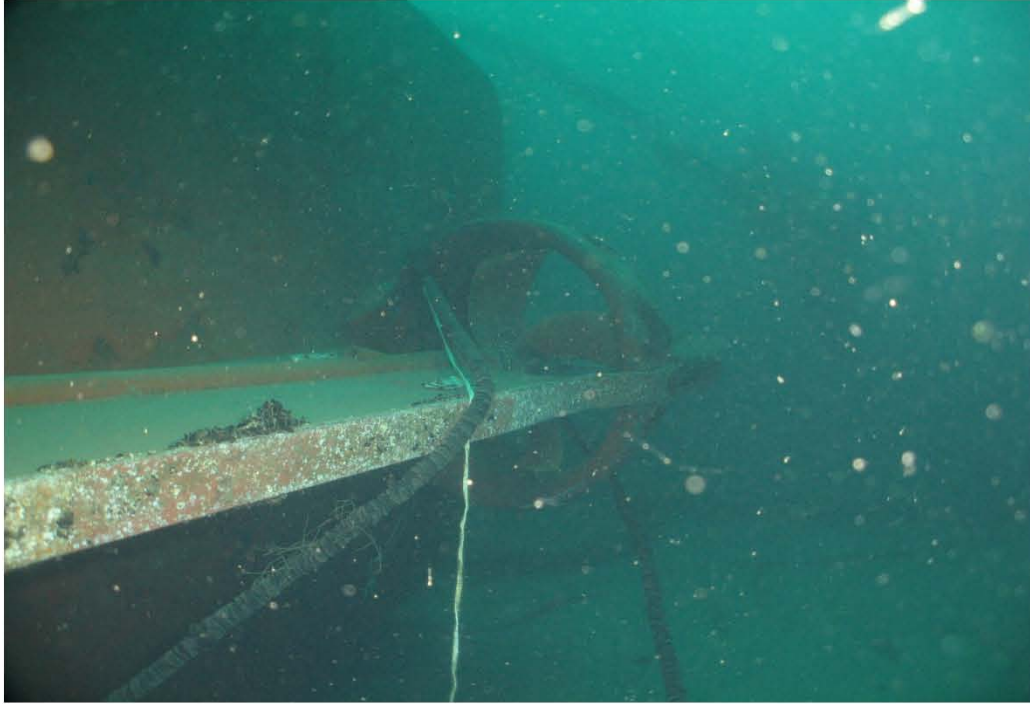
Figure 13: ROV Photo of F/V RHLANNON RAE II's fishing gear ground cable looped on the F/V PATRIOT's propeller
