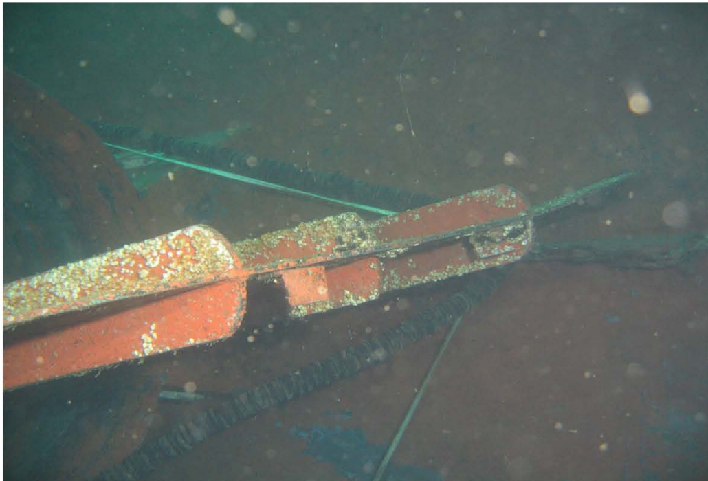
Figure 14: ROV photo of F/V RHLANNON RAE II's fishing gear ground cable and F/V PATRIOT's life raft painter line looped on the F/V PATRIOT's slightly bent rudder
