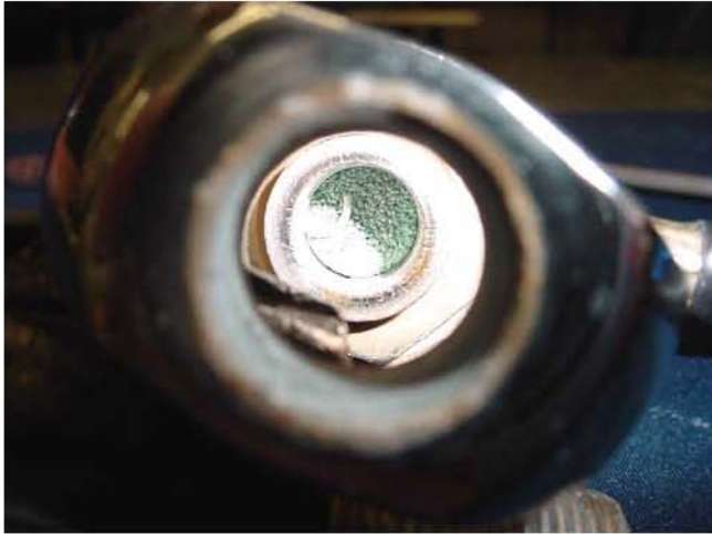
Photo 11: Blue-Green Verdigris encrusted inside 1st Stage Regulator
