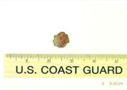
Photo 9: Foreign Object Removed from Regulator (Below)
