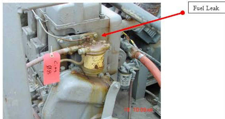
Photo 5: Location of Fuel Leak on Main Compressor
