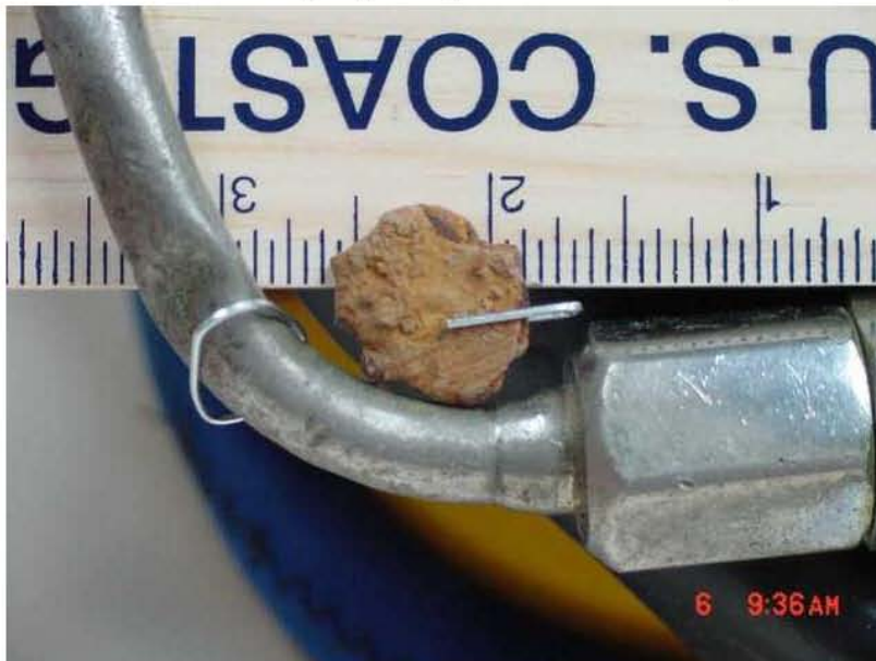
Photo 13: Foreign Object Compared to Bent Tube Assembly
