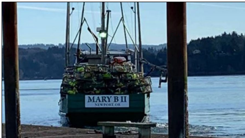
Figure 24. Image of the MARY B II leaving the dock in Newport, OR with crab pots and gear on the after deck prior to the accident voyage. Date is unknown. (Source – Lincoln City Homepage)
