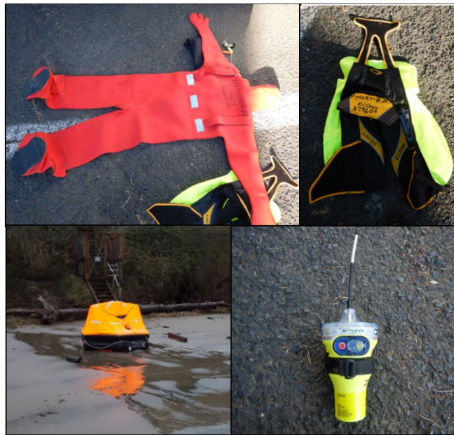
Figure 30. Composite image of MARY B II's safety equipment. Showing an immersion suit, inflatable lifejacket, liferaft and an EPIRB distress device recovered after the accident. (Sources – Mr. [REDACTED] and Oregon State Parks)
