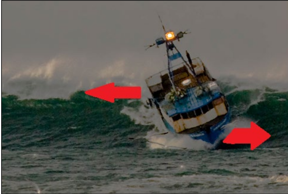
Figure 75. Labeled image of the F/V NORSKEN FISHER entering Yaquina Bay Bar in surf on an unknown date. The red arrows, which have been placed on the image, indicates the dangerous potential for movement of the vessel. Than can lead to broaching if there is a loss of control or an overpowering by the following wave without sufficient power and control to swiftly counteract this momentum. This broaching would result in the vessel laying sideways in the trough of the wave, which most likely lead to a capsizing of the vessel. (Source - Mr. and Mrs. [REDACTED] ©)
