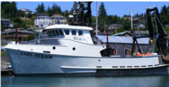
FV LAST STRAW on the left (75 feet in length) in comparison to the FV MARY B II (42 feet in length). Note the high bow and lack of outriggers on the FV LAST STRAW. Images are scaled to show the approximate size comparison and the FV MARY B II image is approximate in size.
