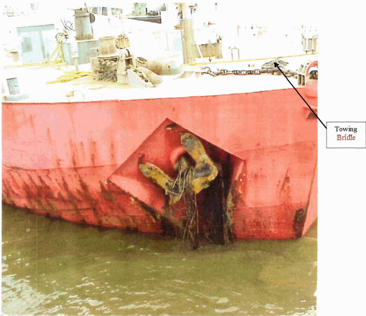
Cement barge MARIA T moored on August 8, 1999. Anchor shows debris picked up as the anchor dragged along the bottom of the Hudson River. Photograph taken August 8, 1999 in Roseton, New York. (Exhibit 54)
