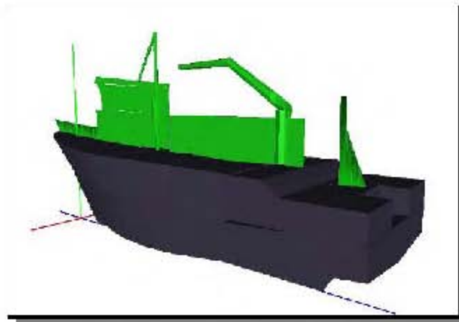
Figure (4). KATMAI 3-D Model for Stability Analysis
