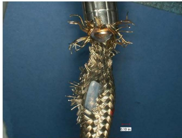
Torn Teflon Liner of Inflation Hose
