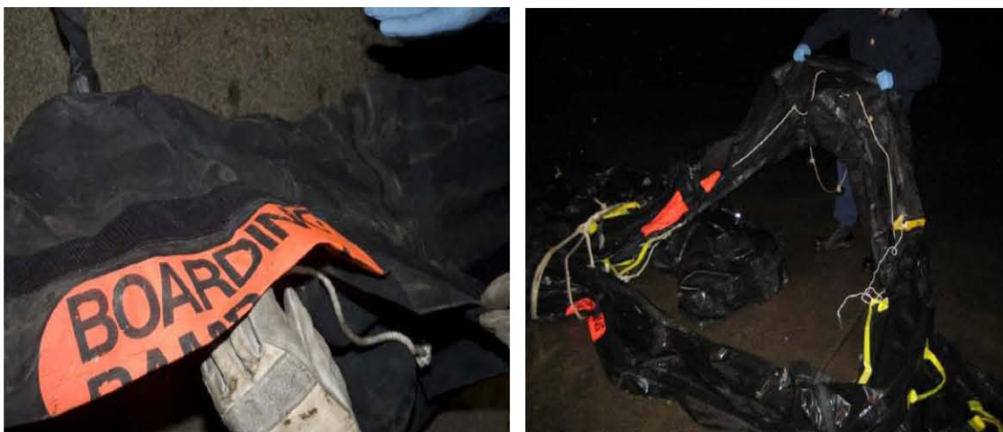
Recovered Crewsaver Liferaft Hull
