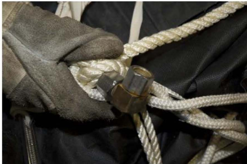
Figure 2. Close-up of the CO 2 inflation hose fitting, which is typically connected to the inflation valve and CO 2 tank.
