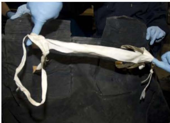
Recovered Lifteraft Gas Cylinder Harness
