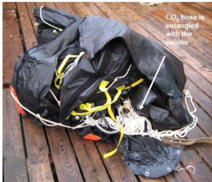
Figure 1. The un-inflated Katmai life raft as recovered on fishing vessel Courageous . The painter is a rope line that attaches the raft to the vessel and when pulled, it activates the inflation mechanism.
