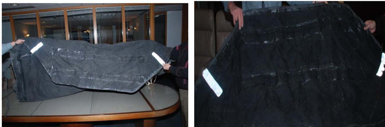
Missing Ballast Bags on Bottom of Liferaft Floor
