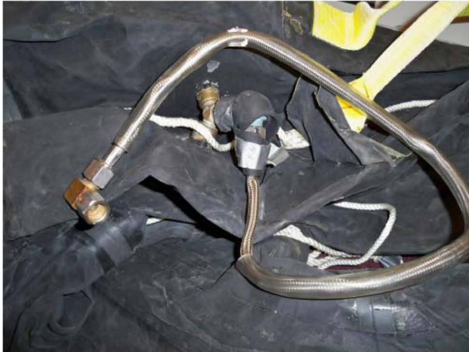
Figure 3. Image of the CO 2 inflation hose attached to the life raft fitting (painter is removed). No CO 2 tank was found with the life raft.
