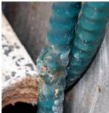
Figures 42 (left) and 43 (right): Photos of Lifeboat No. 8 forward control cable. Credit: CG and DNV-GL.
