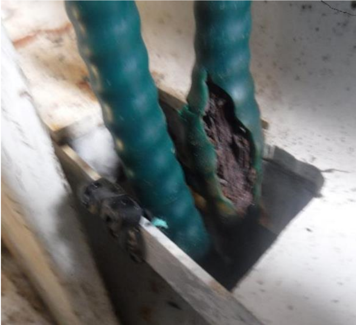
Figure 35: Photo of Lifeboat No. 6 aft control cable. Taken on June 6, 2019. Credit: Palfinger.
