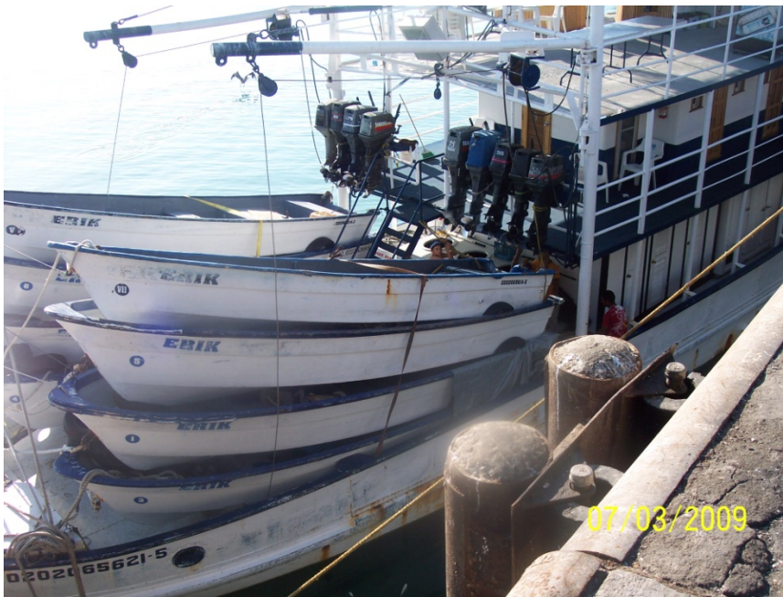
Figure 4: Picture dated 7/3/2009 showing two stacks of “pangas” on the stern of the vessel. This picture was taken before the modifications to enlarge the main deck to accommodate a higher number of “pangas”, and the placement of a fuel tank for their engines.
